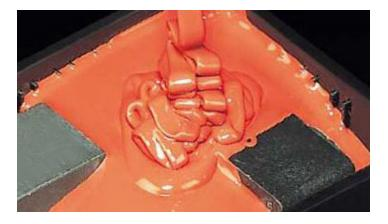
Figure 1. Applying a Thermal Potting Compound.
